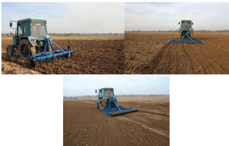
a - improved chisel cultivator; b - improved oscillating - tooth harrow; c - improved mala – leveler
