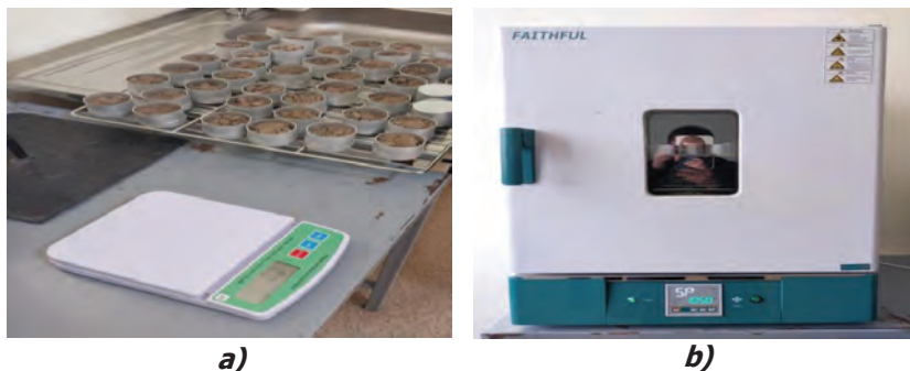
Figure 1. XYSCALE FA2204 model analytical balance a) and WGL - 1258 Drying Oven thermostat b)
