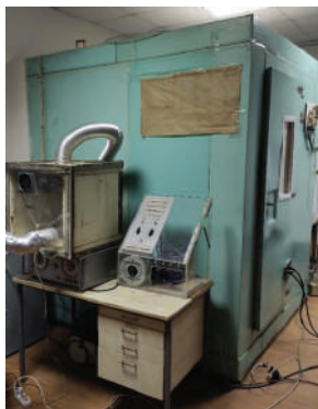
Figure 2 - Large cloud chamber of ice - forming properties of reagents
