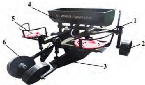
1 - Frama; 2 - base wheel; 3 - planter; 4 - place for seedlings; 5 - seat; 6 - thickness wheel.
